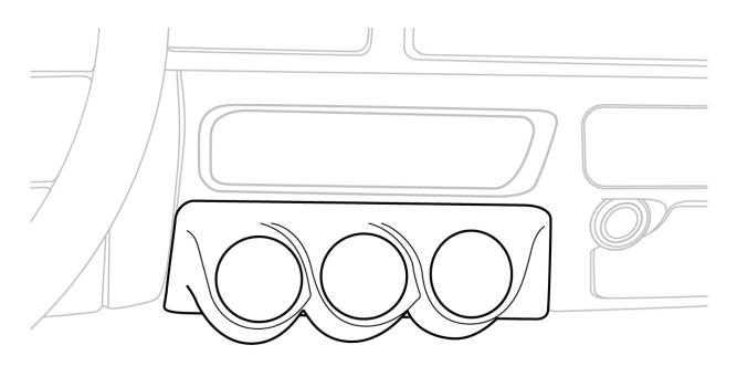
**Note:** This Under dash gauge pod will only fit trucks with an automatic transmission.
