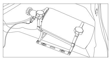
There are a few different ways to connect a Nitrous Pressure Gauge to your vehicle. In most cases an adapter is needed to adapt the 1/8-27 NPT Sensor to your system.
