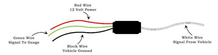
Note: This Tachometer Signal Filter is only compatible with GlowShift and MaxTow brand Tachometers.
