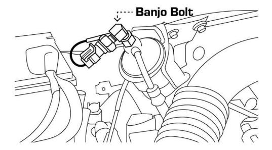
1. Remove the stock banjo bolt from the top of the fuel filter housing using a 17mm wrench.
