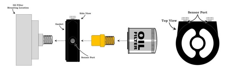
This AF7 Oil Filter Sandwich Adapter is designed for spin on oil filters with a max gasket outer diameter of 4 inches and a minimum inner diameter of 3 inches.
