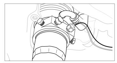
• **T-Fitting Installation:** Remove your stock oil temperature sensor and fasten a T-fitting in its place. 1/8-27 NPT T-Fittings are available for purchase at www.GlowShift.com. Using a T-fitting allows you to "T" off of the port and open up 3 more, which then allows for the stock and GlowShift sensors to be installed and operate simultaneously. Be sure that Teflon tape is being used on the sensor threads.
